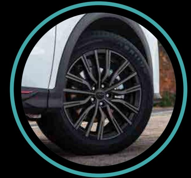
235/55R19 wheels with tyre pressure monitoring system
